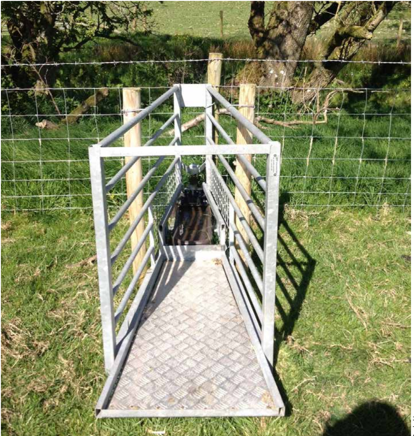
Sheep-operated pasture pump providing water from a fenced-off tributary of the River Ithon in the Wye
